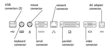
The following table shows the icons for each of the connectors on the back of the APR and indicates the type of external device(s) that you can attach to each connector.
