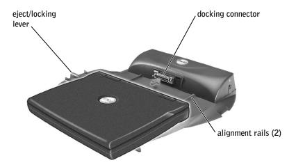
**HINT:** If you have the optional monitor stand installed (see page 13), you will not be able to see the alignment rails or the docking connector.
